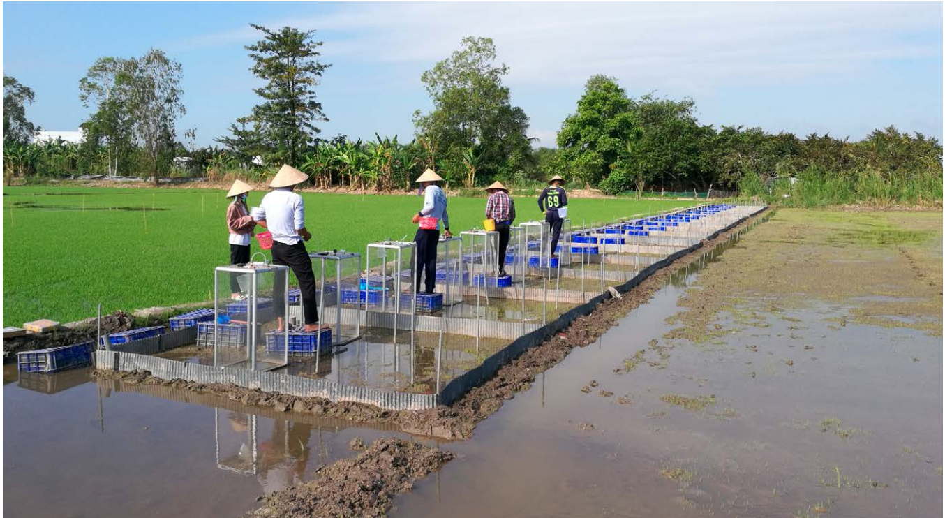
Measurement of GHG emissions from a paddy field in Vietnam
